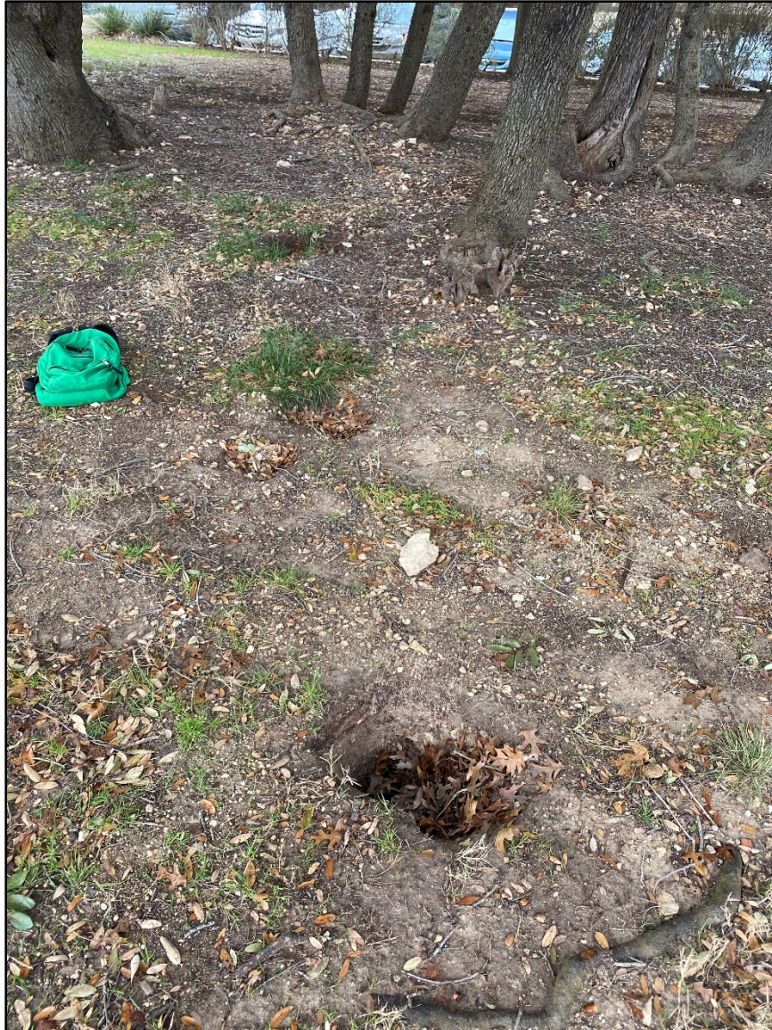
Feature Photo MPS-28 Non-karst Closed Depression. Group of three utility potholes each about 18 inches in diameter. No bedrock exposures were present.
