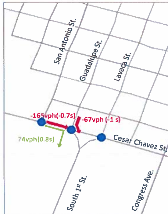
FIGURE 8. CHANGES IN TURNING MOVEMENT AND DELAY PER VEHICLE AT THE MOST AFFECTED INTERSECTION
