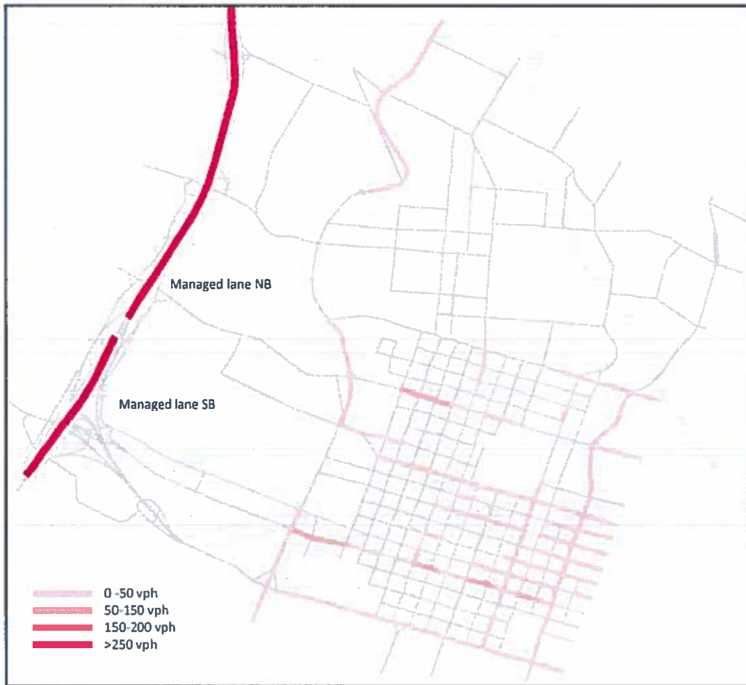
FIGURE 6. LINK FLOW INCREASE IN MANAGED LANES SCENARIO (STREET DIRECTION INDICATED WHEN DIFFERENCES ARE GREATER THAN 150 VPH)
