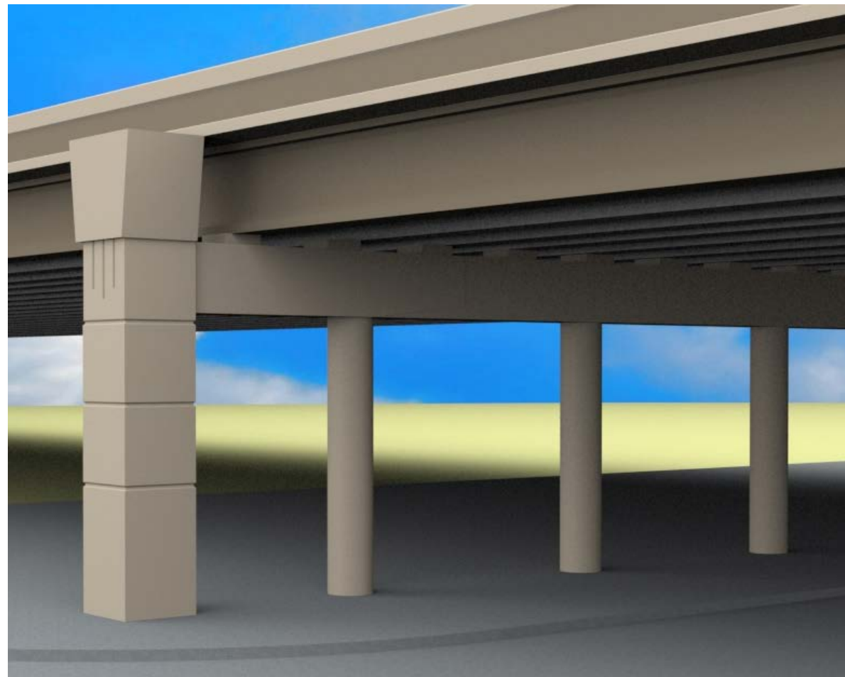
Exterior structural Decorative Column in-line with bent where outside widening of structure. Existing interior cylindrical columns remain Decorative column connected to new cap
