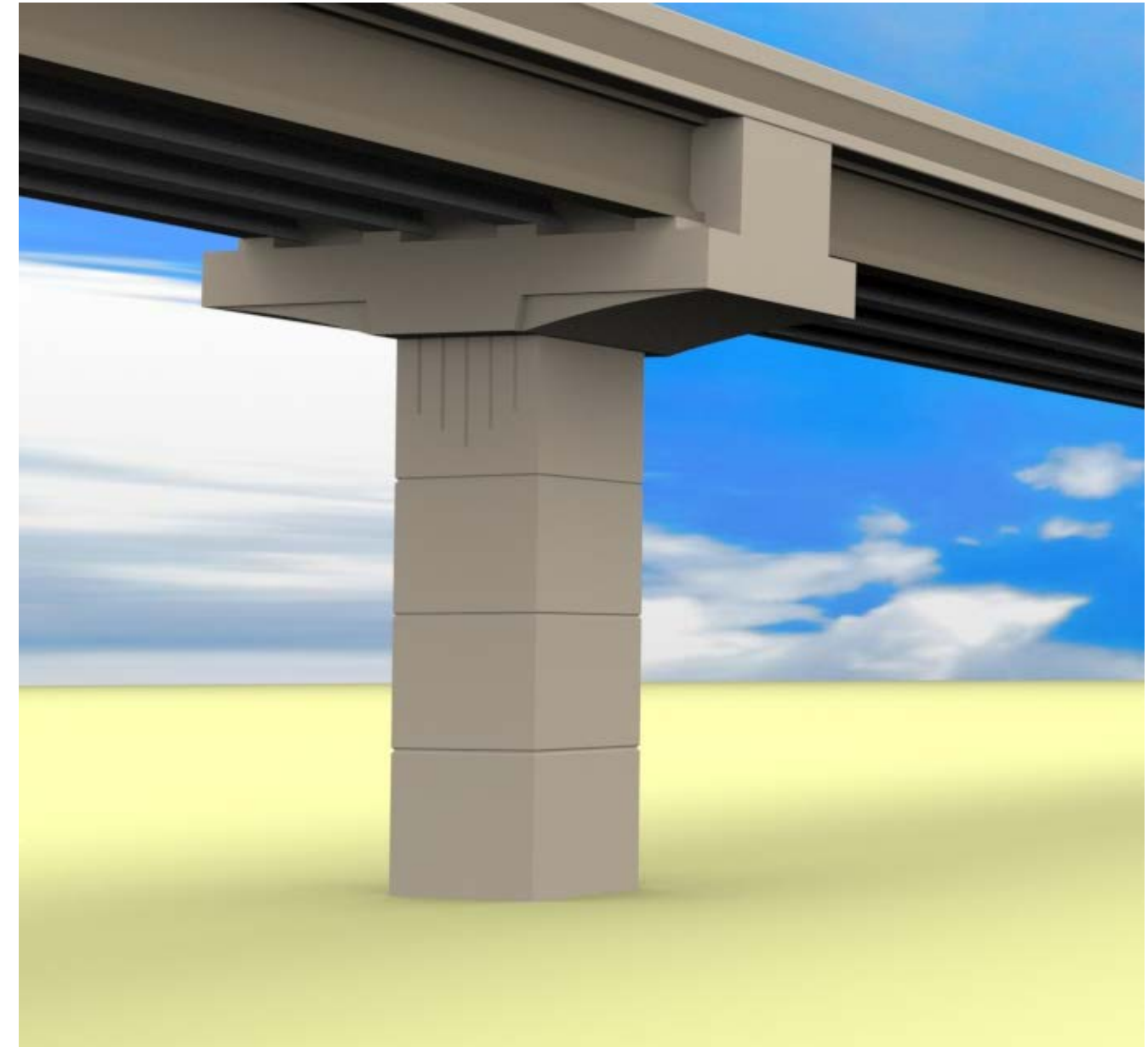
Inverted "T" - Symmetrical Hammer Head – Single Structure
