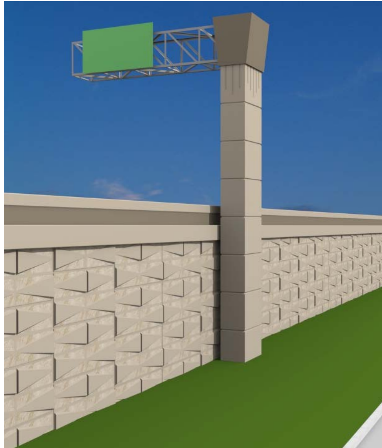
Major Guide Sign / ITS Support Structure
