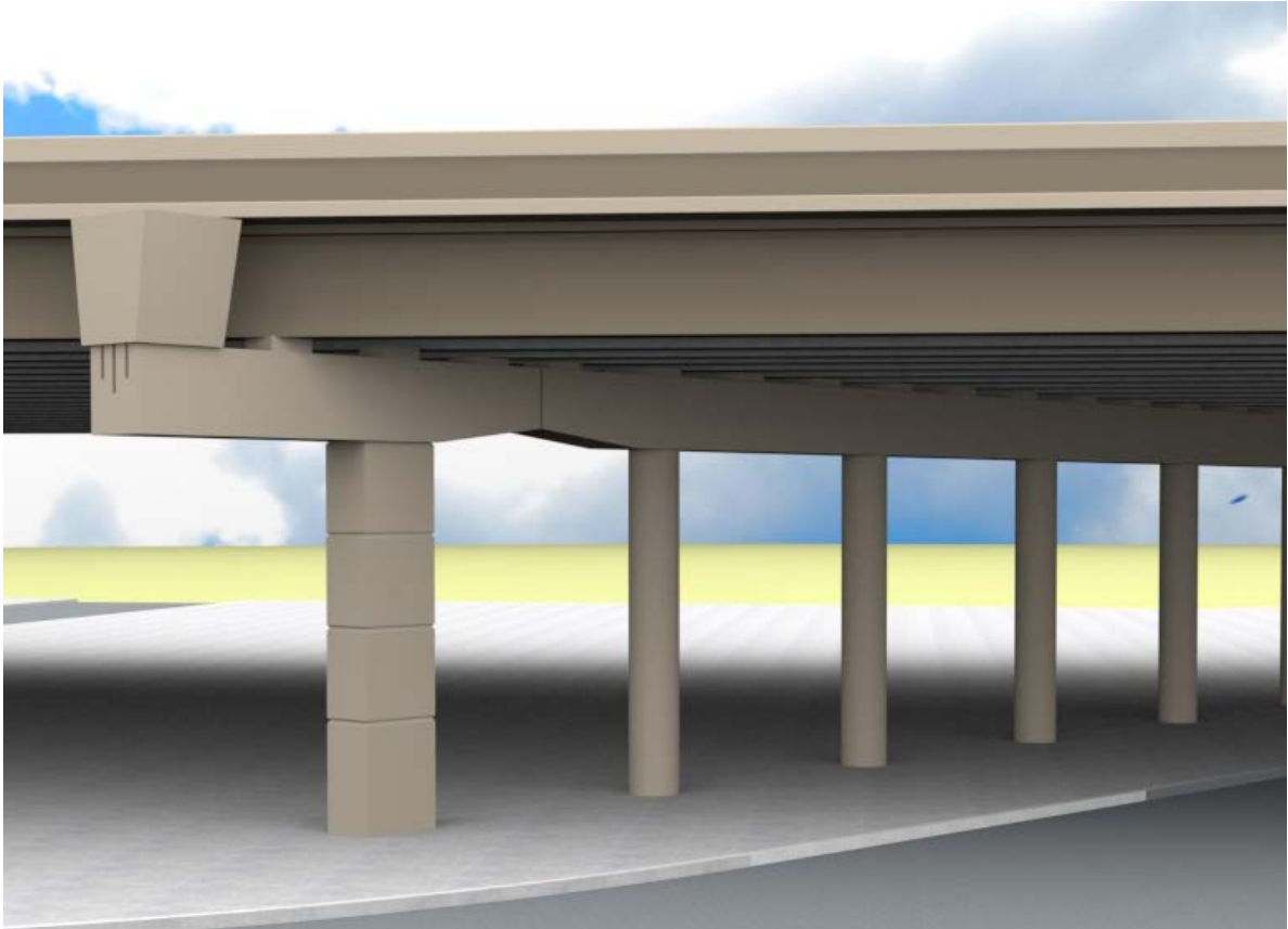
Widening where decorative column is not possible provide extended Cap, Cap Ear Wall and decorative column - Skewed bent location
