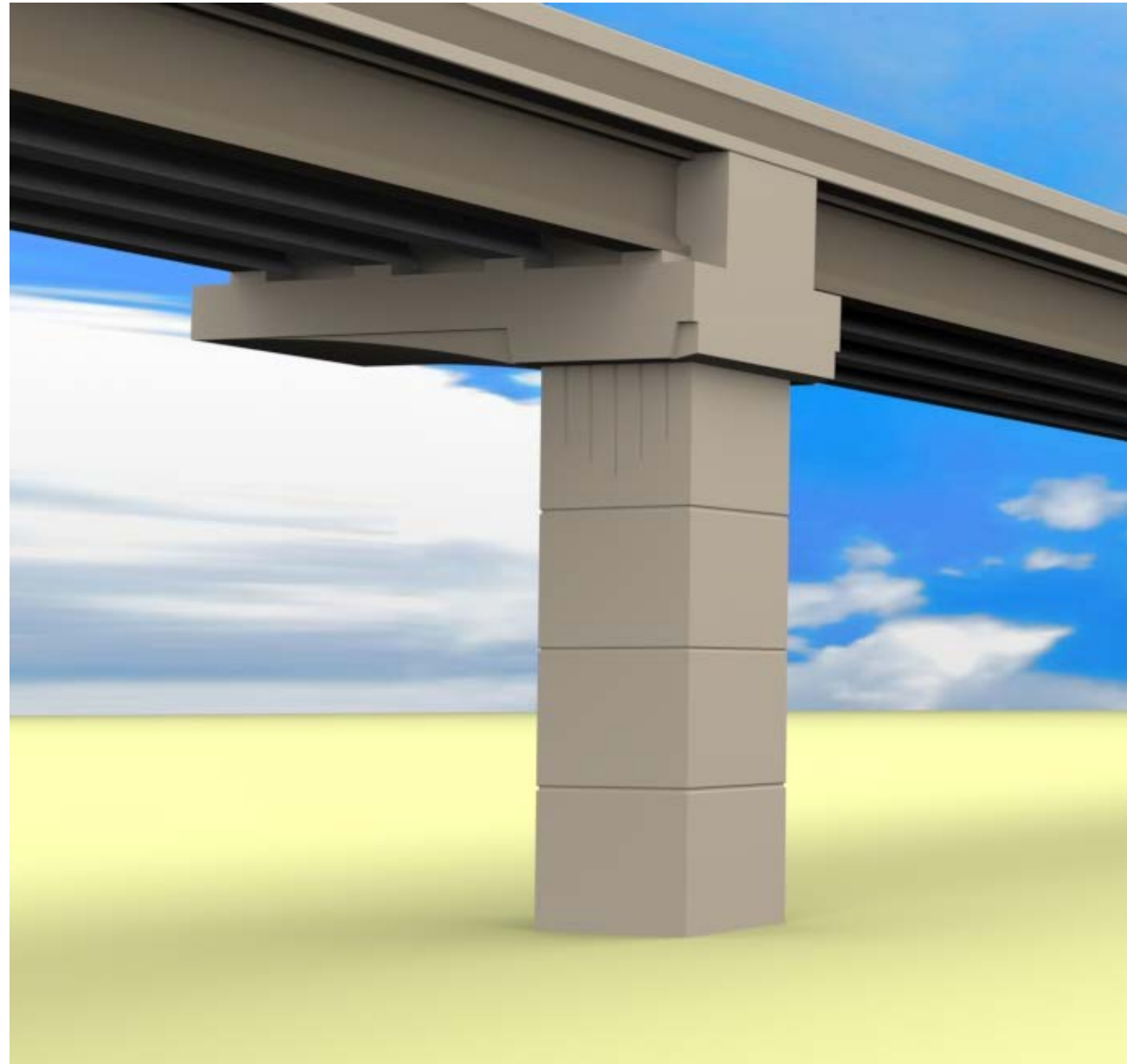
Inverted "T" - Cantilever Hammer Head – Single Structure
